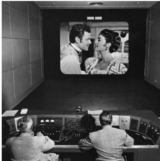
MGM 20-input re-recording console used for most mono films at MGM from early 1940s to 1970s. Only patched EQs on left and right side of console were present.
