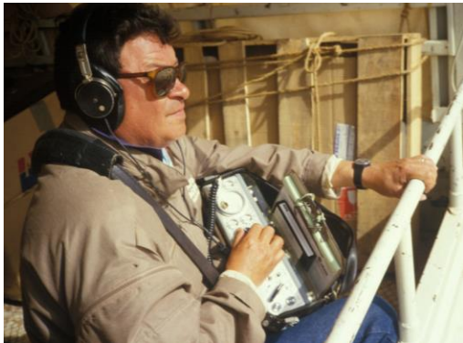
Early 1970s location recording with battery-powered Nagra tape recorder. Photo: Nagra Audio
