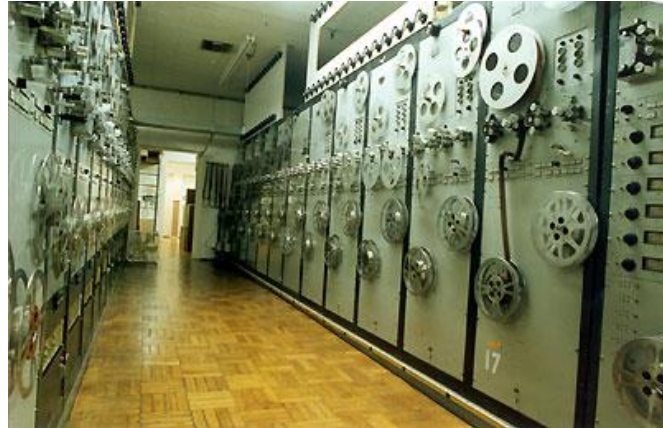
Left: Todd-AO machine room showing the 6-track Westrex mag machines installed in 1950s for 6-track stereo and capable of a total of over 100 tracks. Right: Todd-AO machine room in 1994 shown with Magna-tech dual mag dubbers. Dual-dubbers increased the max track count to around 132. In practice, a mix of single-stripe, 3-track, and 6-track mag units were used so actual track count used would never be that high and was essentially limited by the number of inputs on the re-recording console. Left Photo: unknown, Right Photo: Thomas Hauerslev
