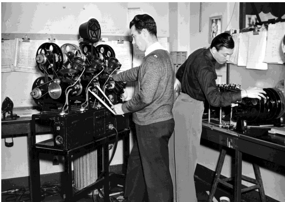
Sound editing at RKO in 1937 showing synchronizer on right and Moviola editor on left. This version allowed three tracks of audio to be synchronized with a work print. Photo: Bison Archive
