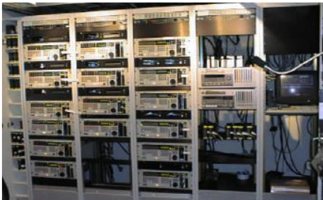
Example of the early 2000s digital dubbers (Tascam MMR-8) that replaced mag machines. This picture shows 128 tracks plus 16-track of DA-88s. The left side shows a shelf of removable hard drives from this era that were often deleted and reused after a mix. Final delivery was on MO Discs or DA-88s. Any mags in this era are typically archival backups of digital elements. Photo source unknown.
