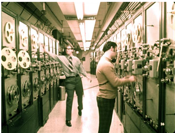
Left: Todd-AO machine room showing the 6-track Westrex mag machines installed in 1950s for 6-track stereo and capable of a total of over 100 tracks. Right: Todd-AO machine room in 1994 shown with Magna-tech dual mag dubbers. Dual-dubbers increased the max track count to around 132. In practice, a mix of single-stripe, 3-track, and 6-track mag units were used so actual track count used would never be that high and was essentially limited by the number of inputs on the re-recording console. Left Photo: unknown, Right Photo: Thomas Hauerslev
