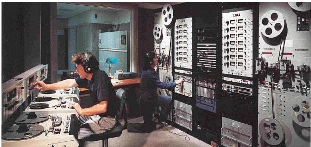
Example of a 1980s machine room recording sync tape dailies and source music tapes to mag film. Typically, 35mm mag film was used for films shot on 35mm film while 16mm magnetic film for used for films shot on 16mm film. Photo: unknown.
