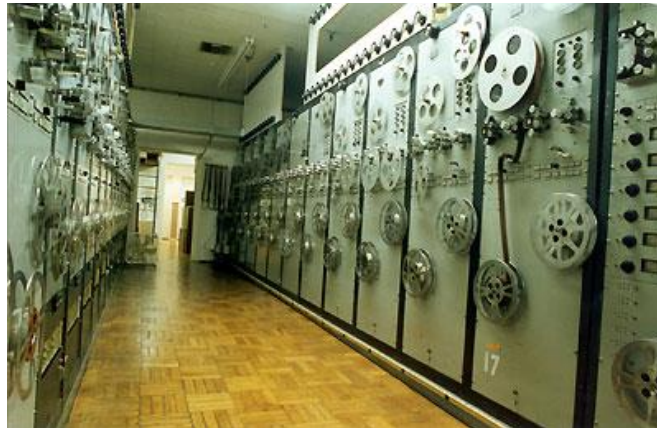
Left: Todd-AO machine room showing the six-track Westrex mag machines installed in 1950s for six-track stereo and capable of a total of over 100 tracks. Right: Todd-AO machine room in the late 1990s shown with Magna-tech dual mag dubbers. Dual-dubbers increased the max track count to around 132. In practice, a mix of single-stripe, three-track, and six-track mag units were used so actual track count used would never be that high and was essentially limited by the number of inputs on the re-recording console. Photos: unknown
