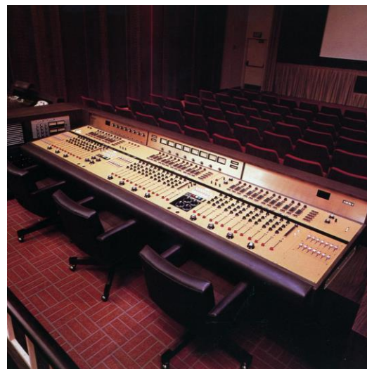
Quad-Eight console at Goldwyn used for Star Wars (1977) mix. Modern-era consoles with EQ on each channel and buss assignments were not used for film sound until the 1970s or even early 1980s at some studios. Photo: Quad Eight catalog
