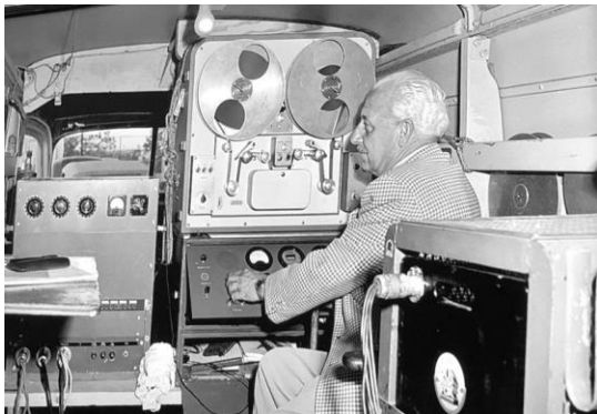
Example of production mag recording equipment being used within a sound truck similar to the earlier optical recording systems. Photo: Courtesy of the Academy of Motion Picture Arts and Sciences
