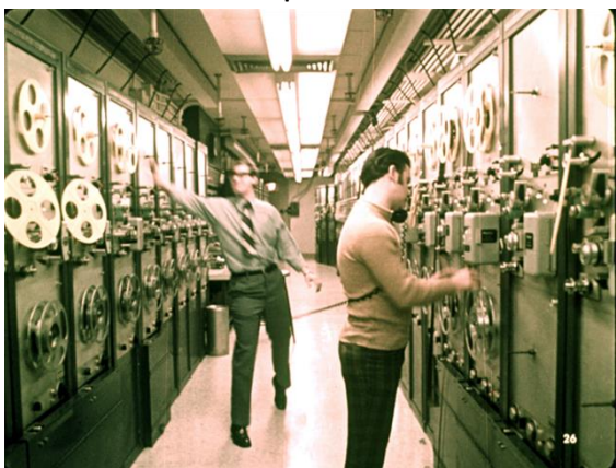
Left: Todd-AO machine room showing the six-track Westrex mag machines installed in 1950s for six-track stereo and capable of a total of over 100 tracks. Right: Todd-AO machine room in the late 1990s shown with Magna-tech dual mag dubbers. Dual-dubbers increased the max track count to around 132. In practice, a mix of single-stripe, three-track, and six-track mag units were used so actual track count used would never be that high and was essentially limited by the number of inputs on the re-recording console. Photos: unknown
