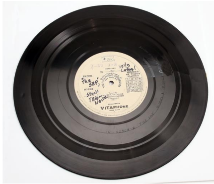
Example of an original Vitaphone source recording of train effects used as a mix unit. This element would be placed on one of the turntables shown in the earlier disc machine room image.
