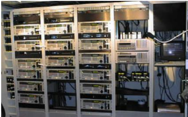
Example of the early 2000s digital dubbers (Tascam MMR-8) that replaced mag machines. This picture shows 128 tracks plus 16-track of DA-88s. The left side shows a shelf of removable hard drives from this era that were often deleted and reused after a mix. Final delivery was on MO Discs or DA-88s. Any mags in this era are typically archival backups of digital elements. Photo: unknown.
