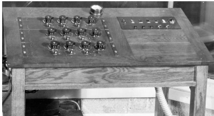
1928 Modular Western Electric mixer capable of any number of inputs and groups by adding panels as desired. By March 1928 they were already specifying nine inputs and two group outputs. The version on right is similar but uses three output groups (right-most knob on each of the panels). Photo: Endpoint Museum collection
